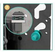
**Spring loaded mounting studs** push cabinets into the final Z-axis position.
