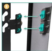
Magnetic trim is attached using alignment pins and held in place with powerful rare-earth magnets, making installation or removal quick and easy.
