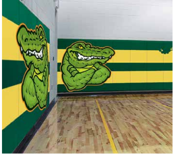
Wall pads, while providing protection with low VOCs, can also serve as a design element with custom printing available.
