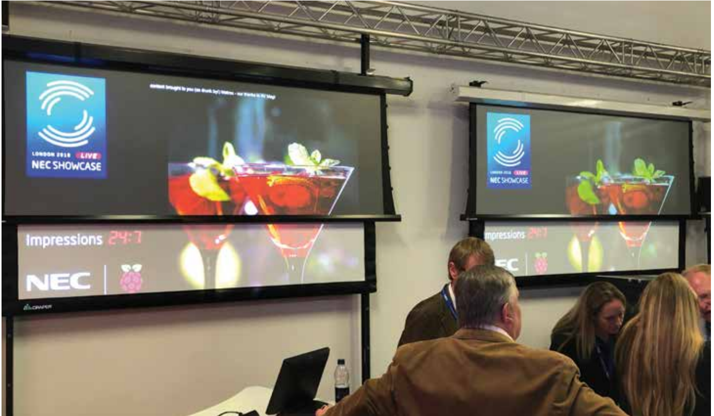
Visual examples of screens in ambient light, TOP: ALR screens , BOTTOM: Non-ALR screens
