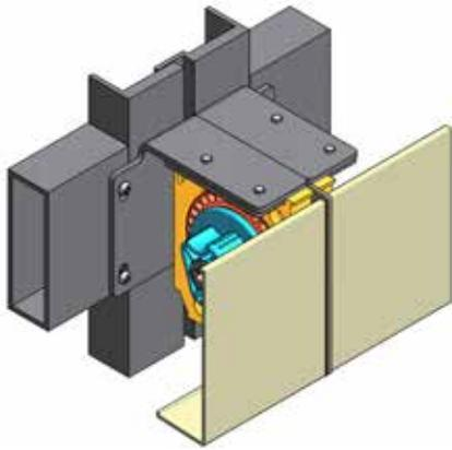
Based on a detail drawing of the horizontal mullion, Draper engineers produced a 3-D drawing of a custom bracket. After some feedback the design was slightly modified and approved.
