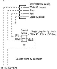
NOTE: Test shade operation. If shade direction does not correspond with the switch orientation, turn power back off and switch the red and black wires from the motor to the switch.
