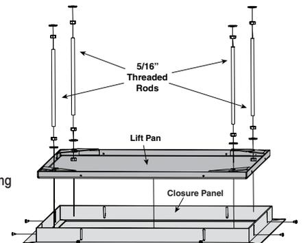
**Please Note:** Immediately upon completion of the surrounding ceiling, units should be operated to confirm that optional ceiling closure panel stops just short of touching ceiling in closed position.
