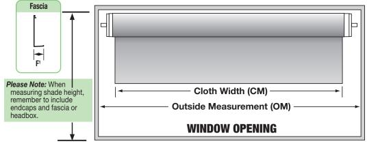
Overall Width includes plastic endcap covers) (Pair adds 1/8" to Overall Width)
