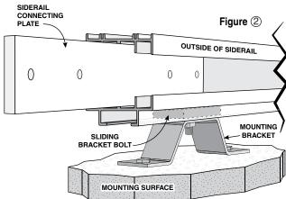
Align the pre-drilled holes and attach provided nuts.
