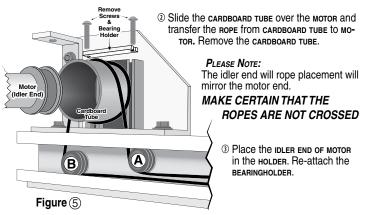
You are now ready to install the roller assembly into the TOPSPIN SIDERAILS.
