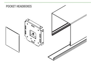
The Pocket-Style Headbox features an extruded aluminum headbox with endcaps for ceiling-recessed installation of a single roller shade. In case you need to pre-install a headbox, we recommend using the Type D Pocket. The Pocket-Style Headbox is not designed for pre-installation as the shade must be installed at the same time as the headbox.
