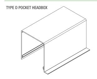
Extruded aluminum headbox with tile lip for acoustical ceiling support. If product fits into large hardware, it will fit into the Type D Pocket. Stock Length 147". White finish only. Use 1-1/2" removable closure panel with manual shades and 3" closure with motorized shades.
