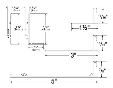
Wall clips for mounting closure panels in existing pockets. Known in specs as "no cost pockets". Clips are available with or without tile lip for acoustical ceiling support. Aluminum extrusions are 147" stock length. Can be cut to size by Draper or by dealer. Compatible with closures listed below. White finish only.
