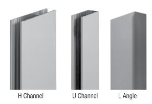
Aluminum side and sill channels for light gap reduction. U and H Channel are 195" stock lengths. Small 1" L Angle is 147" stock length. Large 2 3/4" L Angle is 195" stock length.
