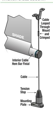
Interior cable guide kit uses a 5/8" round hembar in an open ended pocket. Kit includes all options for wall or deck mounting and is compatible with brackets or endcaps and fascia. May be used on slightly sloped facades.
