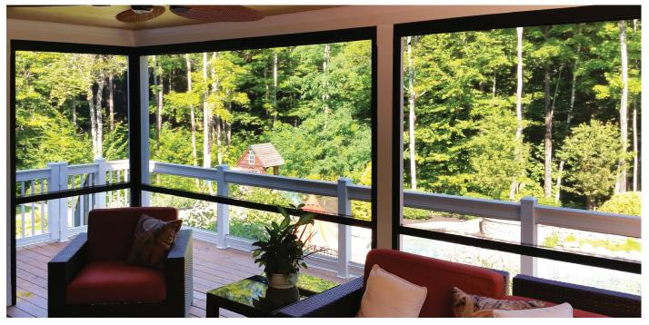
The FlexShade<sup>®</sup> ZIP exterior shading system prevents heat from entering a building, thus lowering HVAC costs. In outdoor covered spaces—such as garages, porches, or commercial food service areas—it keeps harsh glare out, providing a more comfortable environment. The zip detail in the shade stops the fabric from being pulled out of the side channel. The shade system protects against wind and insects, creating a more pleasant outdoor experience.
