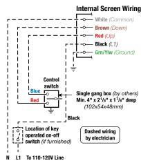
Ropewalker Wiring for Low-voltage Control
