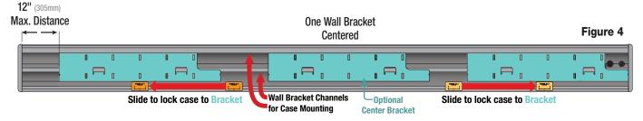
5. Once the case is settled on the mounting brackets, slide the Bracket Locks to the center of each mounting bracket (see Fig. 4) and secure set screw on the lock.
