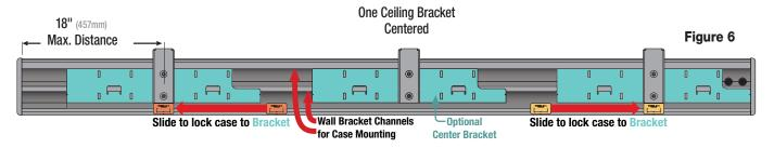
6. Once the case is settled on the mounting brackets, slide the Bracket Locks to the center of each mounting bracket (see Fig. 6) and secure set screw on the lock.
