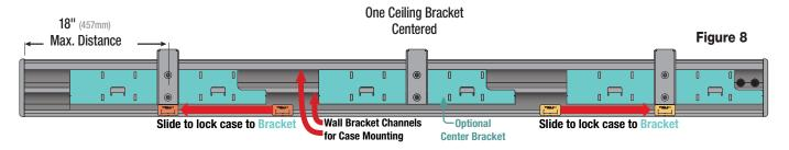
6. Once the case is settled on the mounting brackets, slide the Bracket Locks to the center of each mounting bracket (see Fig. 8) and secure set screw on the lock.
