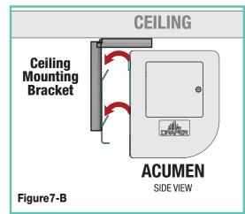
5. Holding the case by the endcaps, lift it up and over the cleats on the mounting brackets (see Fig. 7). Wall Bracket Mounting Channels are shown in Fig. 8 below.
