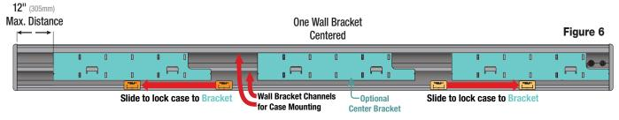
5. Once the case is settled on the mounting brackets, slide the Bracket Locks to the center of each mounting bracket (see Fig. 6) and secure set screw on the lock.
