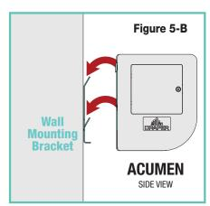
4. Holding the case by the endcaps, lift it up and over the cleats on the mounting brackets (see Fig. 5). Wall Bracket Mounting Channels are shown in Fig. 6 below.
