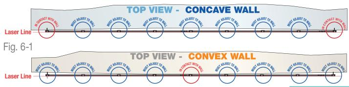
2. For any wall brackets not touching the wall (see BLUE CIRCLES ABOVE) use a 5mm Hex Wrench to loosen the four (4) locking screws on the top and bottom of each bracket (See Fig. 6-2).
