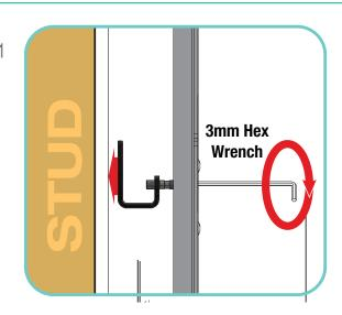
2. Use the clearance hole in the vertical rail to allow for a socket to drive a lag screw (by others) into the wall.
