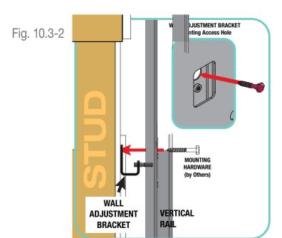
3. Rotate the differential screw to push or pull the vertical rail to be straighter if required.
