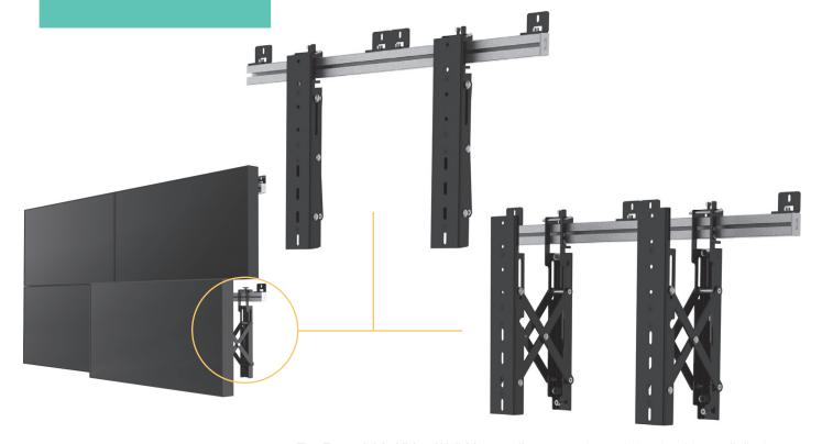
The **Extendable Video Wall Mount** offers a premium solution for video wall display units by providing easy access for service or exchange. Each mount contains a spring-mounted extension mechanism tto move the display out away from the wall. Save time and money by avoiding the necessity of removing the other displays in the array.
