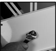
Thread the following: Washer (.375 ID x .875 OD x .064"), Two (2) Long Slotted Arms, Two (2) Short Slotted Arms, and a second Washer (.375 ID x .875 OD x .064") onto the 5/16-18 x 11/4" Machine Screw.
