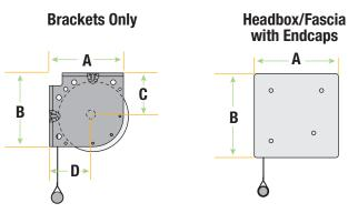
Please Note: Fascia or headbox will add 1/8" between the wall and the bracket; headbox will add 1/16" between ceiling or wall and the bracket.
