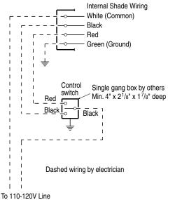
NOTE: Test shade operation. If shade direction does not correspond with the switch orientation, turn power back off and switch the red and black wires from the motor to the switch.
