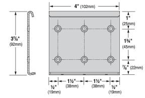
NOTE: Mounting brackets attach to surface with #10 Flat Head Screw
